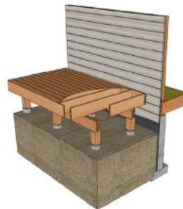
..... Open Deck - Independent Structure (Post Support) .....
