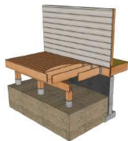
..... Open Deck - Ledger Attachment .....
